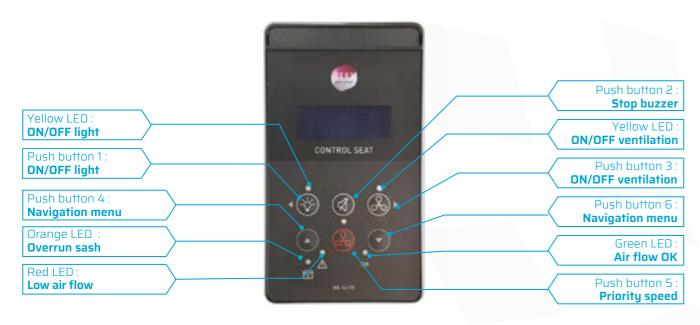
This controller is EN 14175 and HMI Dimensions **CPU Dimensions RoHS** compliant R40 EC1 EC2 EC3 EC4 Configurable dry contacts Configurable relays 0/10V output (SA2) Alarm relay Linear position sensor (EA1) . O/10V output or 4/20 mA (SA1)230V power supply
